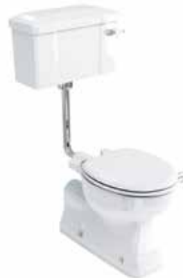
S trap low level WC with 440 lever cistern W: 440 D: 740 H: 1075 Pan: P19 Lever Cistern: C3 Button Cistern: C4 Flush Pipe: T31 CHR
